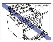
• Do not touch the paper feed roller under any circumstances. Doing so may cause the paper feed mechanism to malfunction.
